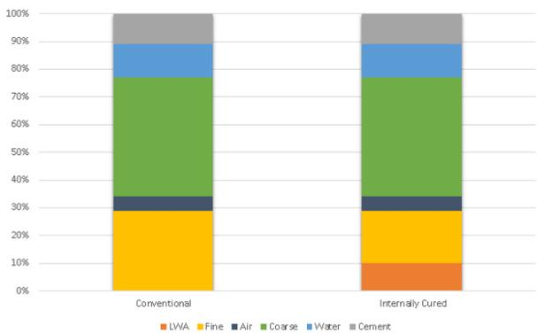
Figure 2. Example of volumetric mixture proportions of both conventional and ICC concrete
