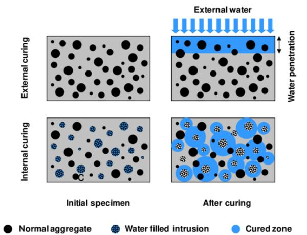
Figure 1. Differences between external curing and internal curing provided by pre-wetted LWAs
