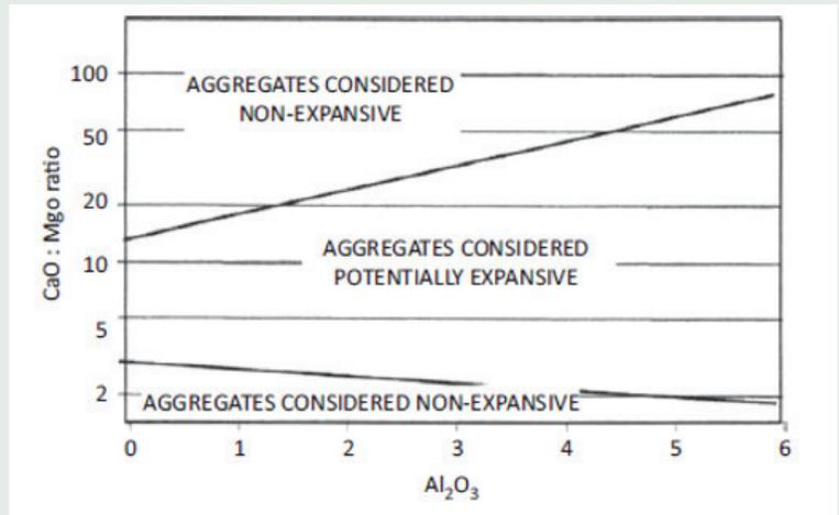
Figure 1. A sample plot of CaO/MgO ratio versus the Al<sub>2</sub>O<sub>3</sub> content of quarried carbonate rocks.
