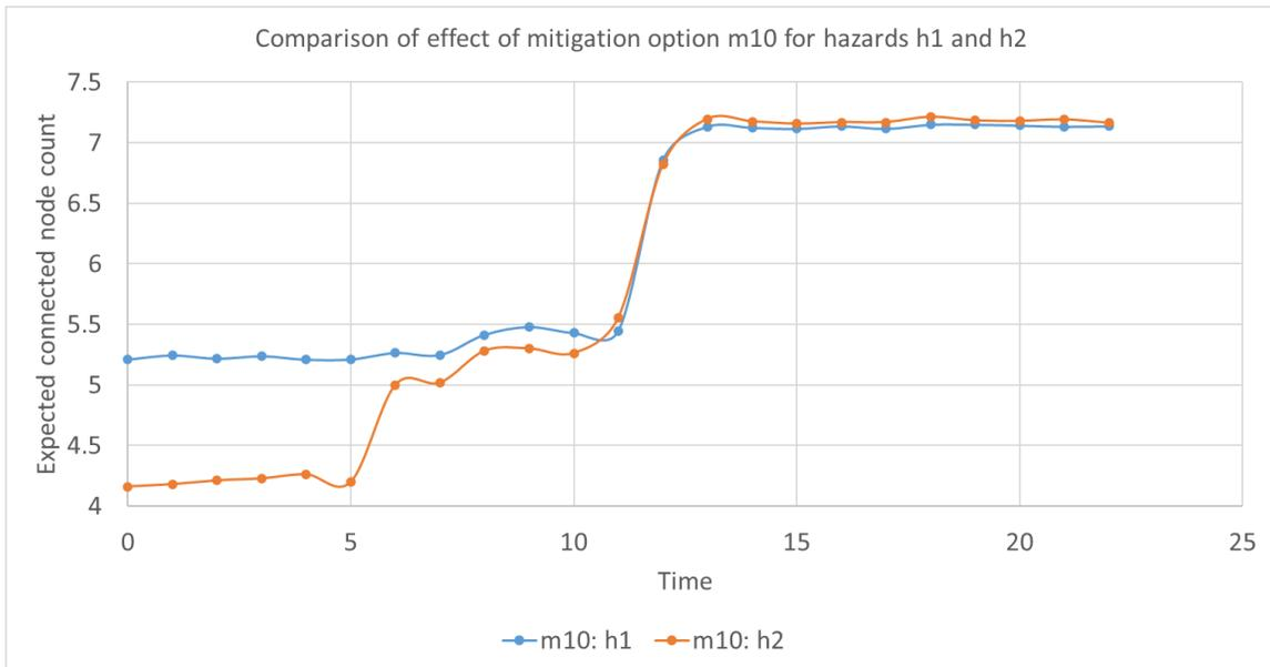
Figure 10 shows the improvement of performance of the network as the tasks for mitigation option m10 are completed. The blue dotted line indicates the expected connected node count at each time step and the black bars indicate the completion of a task. Note that this is displayed for hazard H2. As discussed previously, the tasks are completed at time steps 5, 7, 10, 11 and 12. The improvements in performance are also seen right after the completion of tasks.
