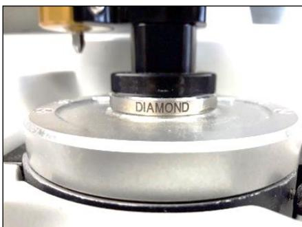
Samples were placed directly on the diamond crystal as shown in Figure 22. Using default software settings (wavenumber range of 4000 to 650  $\text{cm}^{-1}$  and resolution of 4  $\text{cm}^{-1}$ ), 24 scans for each sample were averaged and the resultant spectrum was collected as shown in Figure 23.
