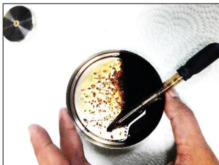
**Figure 19. Filtration technique for HMA mix**
