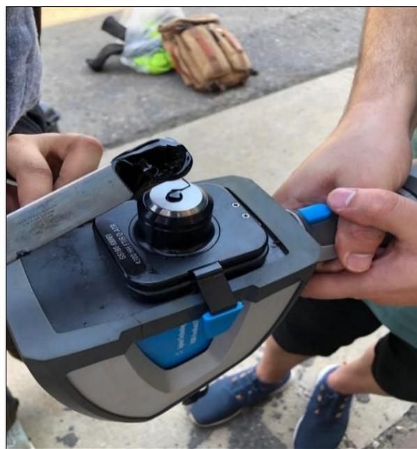
**Figure 12. Ensuring good connection between sensor and sample**
