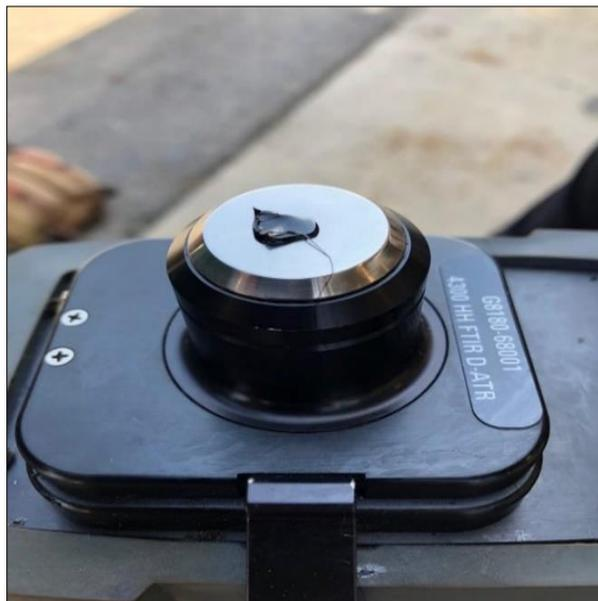
**Figure 13. Collecting FT-IR spectra**
