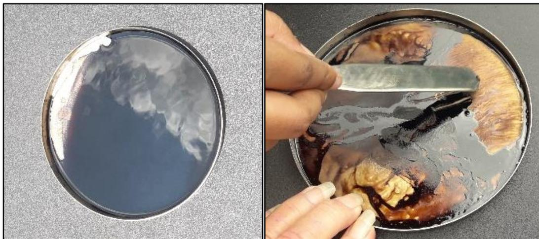
[6] Binder residue is collected using a spatula and placed on the diamond crystal of the FT-IR for recording the spectra.
