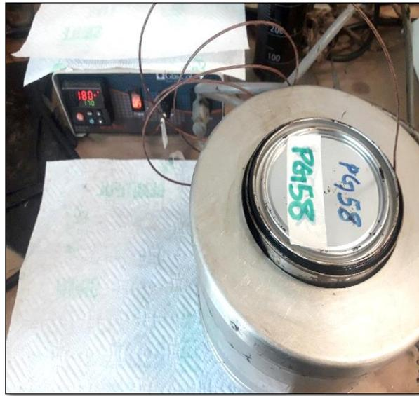
**Figure 2. Adding powdered SBS in the liquid asphalt binder**
