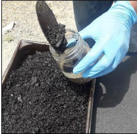
[3] Dichloromethane (DCM) is used as a solvent to extract the binder from the mix. Around 100 milliliters of DCM is poured into the jar containing the loose mix. Immediately after pouring the DCM, the jar should be shaken well for around 30 seconds. After that the jar should be left for five minutes to get the binder dissolved into the solvent.
