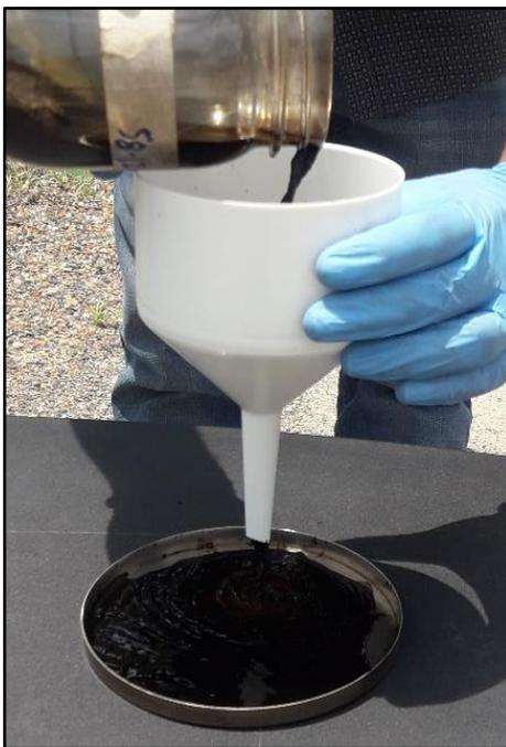
[5] The pan was kept on a table at an open space in the plant. Because the place was open, it was nicely ventilated. Most of the DCM evaporated within five minutes. After five more minutes, 10 minutes after filtration, all the DCM was evaporated and the binder residue was left on the metal pan. The amount of the binder was enough to record the FT-IR spectra for 10 replicates.
