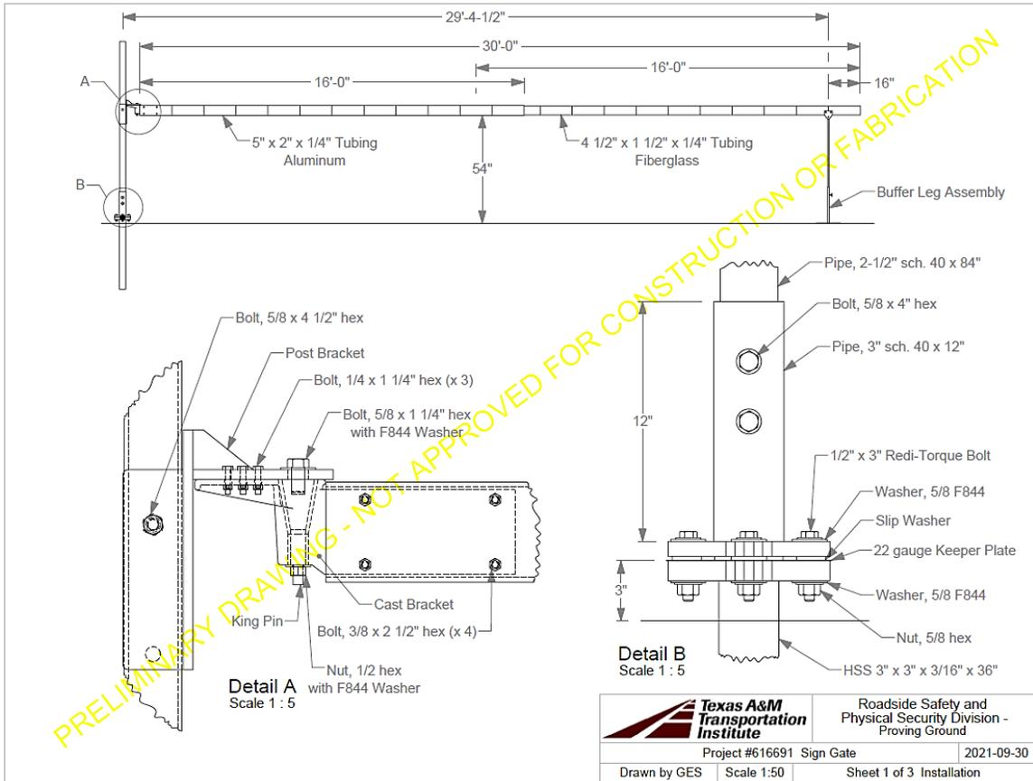
**Figure 4. Contraflow ramp closure gate—post bracket and cast adapter**
