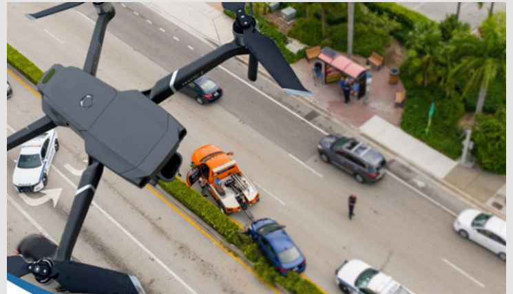
Figure 2. Traffic incident response monitoring with a UAV (Carrick & Burgess, 2021)
