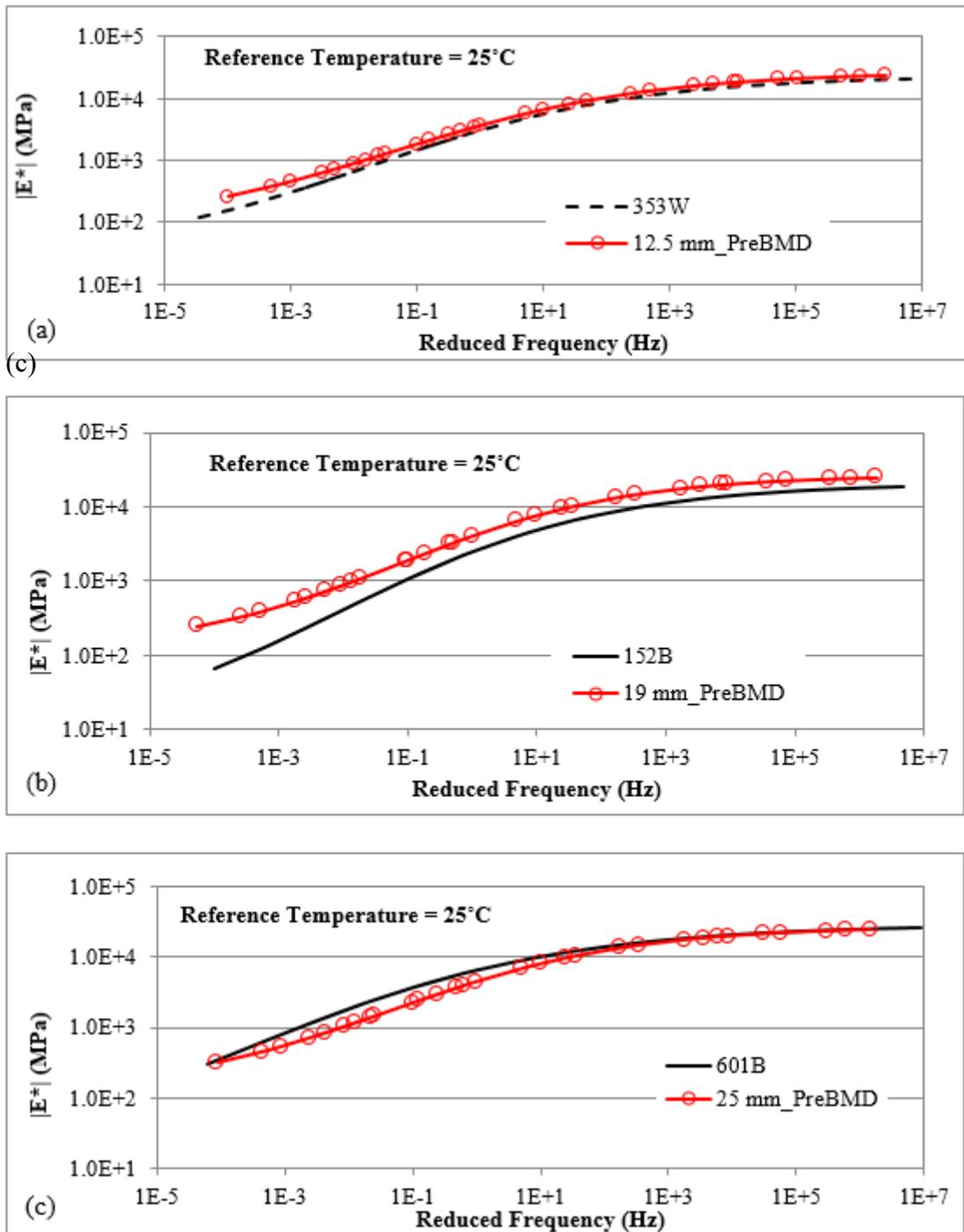
The dynamic modulus values were further analyzed to determine  $|E^*|_{54^\circ\text{C}, 5\text{Hz}}$  parameter of mixtures designed using the current mix design specification compared with their
