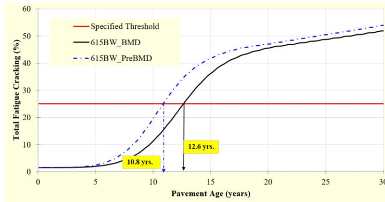
**Figure 14. Pavement ME performance curves for 124BW**
