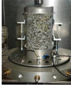
(c) Sample Setup for LTRC  $|E^*|$  test
