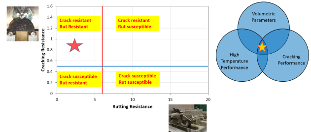
Figure 1. Louisiana DOTD Performance-Based Specification
