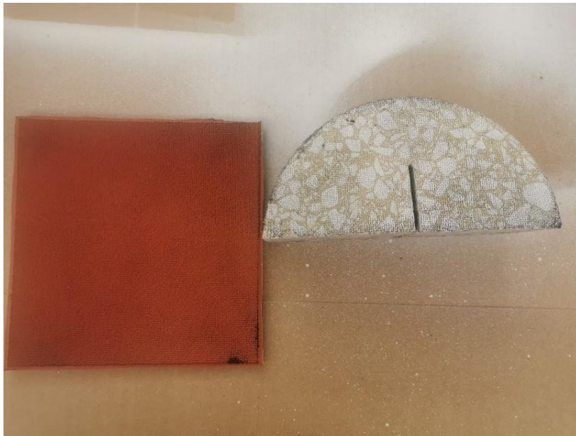
Figure 5. Speckle stamp and SCB specimen with speckle pattern
