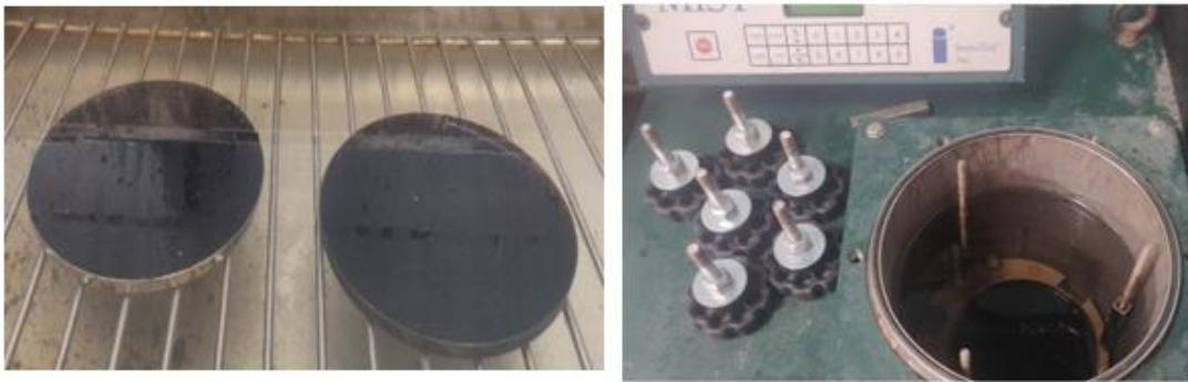
Figure 9. Freeze-thaw and MiST conditioning of asphalt binder samples
