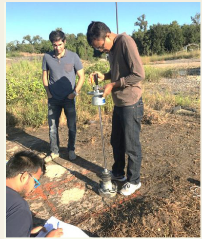
Field testing of soil property using LFWD
