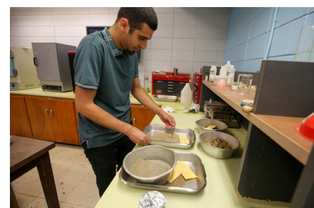
Ph.D. student Isam Khasib preparing a sample to wet sieve it.
