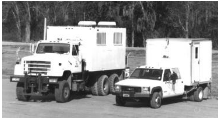
(a) Louisiana cone penetration test systems: the CIMCPT on the right and REGEVITS on the left
