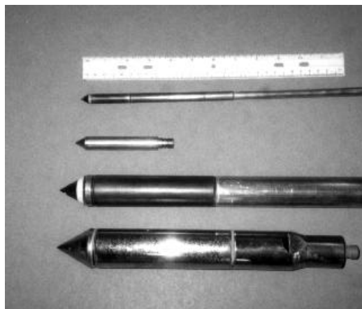
(b) The 1.27, 2, 10, and 15 cm 2 cone penetrometers used at LTRC
