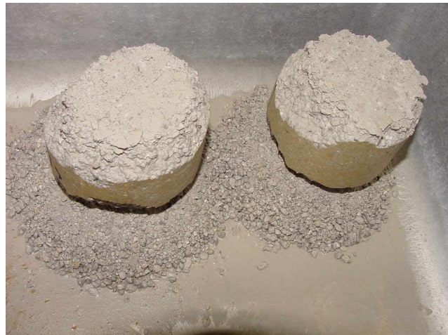
Figure 6-b. Two BCS Specimens after Soaked in Water
