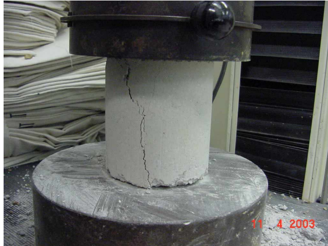
Figure 6-a. A BCS Specimen Tested on Dry
