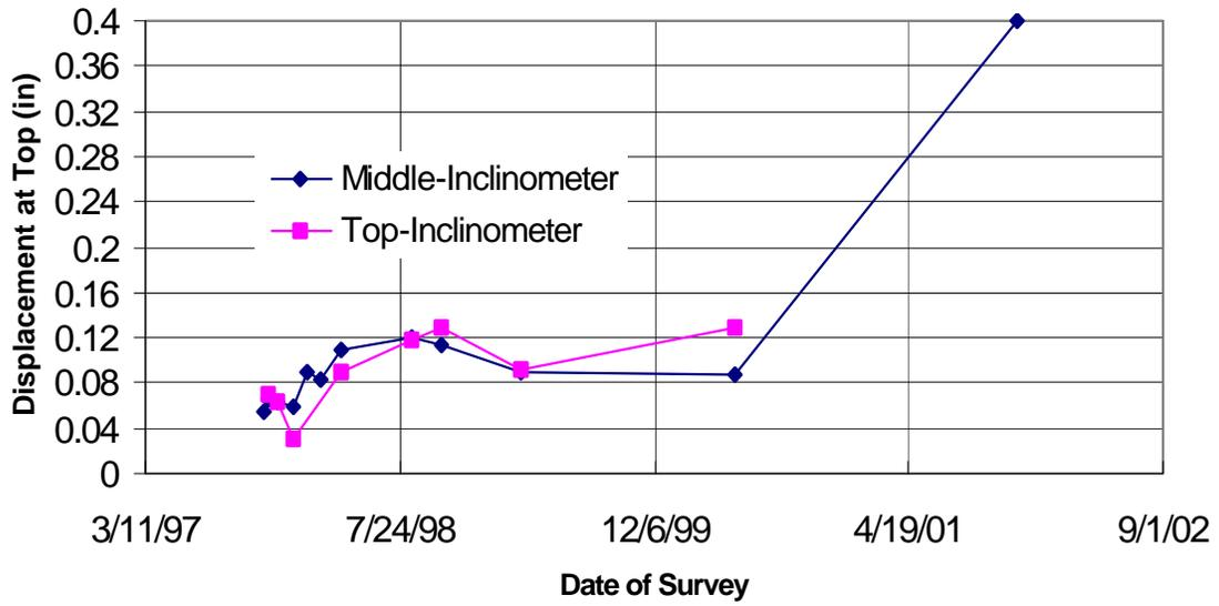
Figure C-10: Time deformation of the inclinometers, section 224
