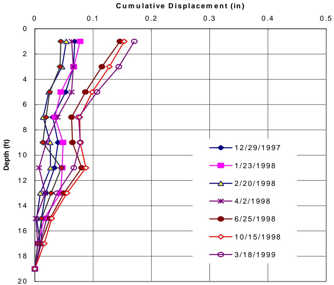
Figure C-11: Top inclinometer readings in section 242 [soil only]
