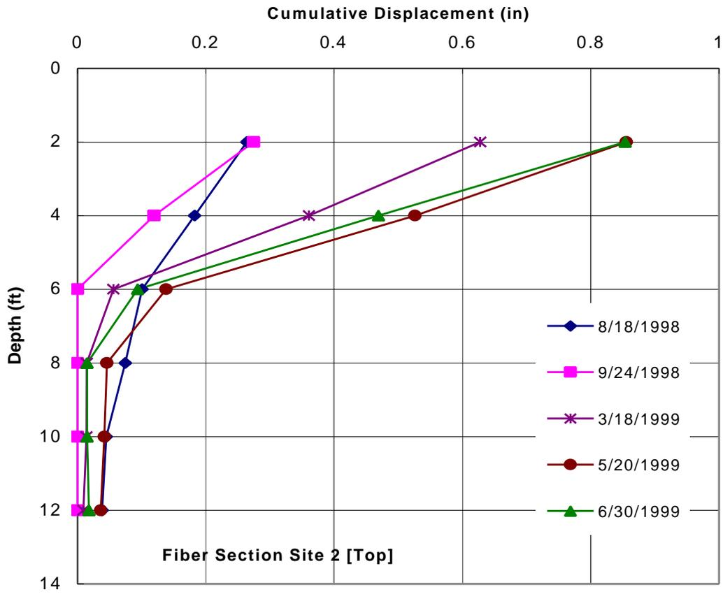
Figure D-4: Readings of the top inclinometer in fabric section 2
