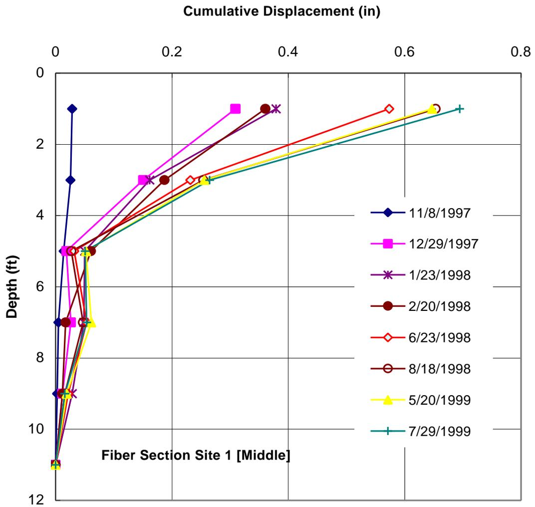
**Figure D-2: Readings of the middle inclinometer in fabric section 1**
