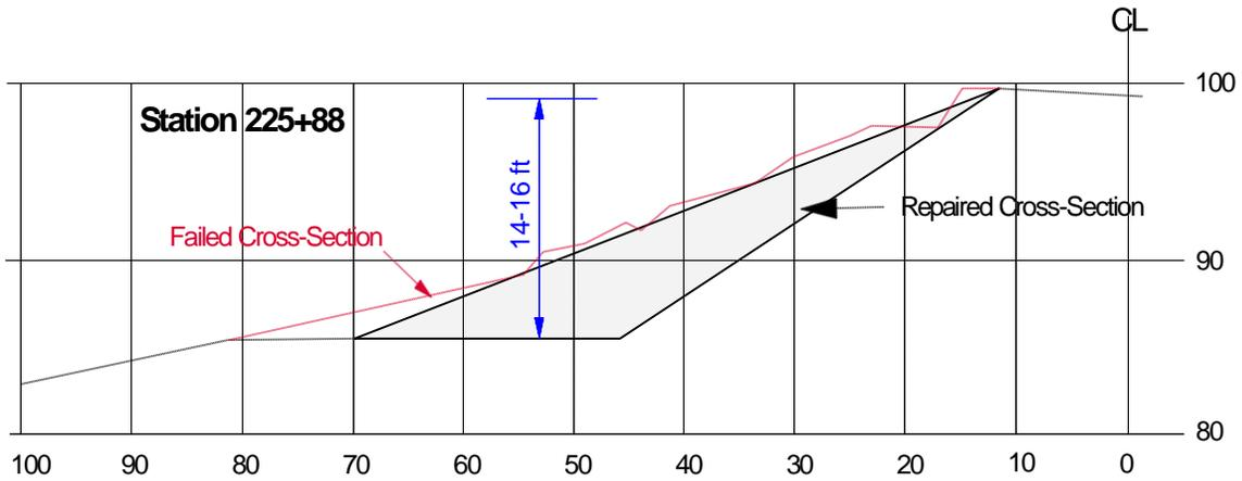
Figure A-5. Typical cross-section of the slope in section 224
