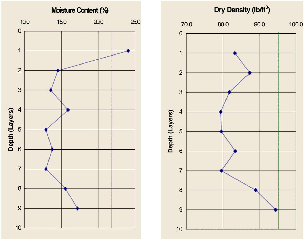
Figure A-6. Field measurements of moisture and density in section 224
