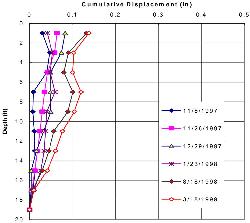
Figure C-14: Top inclinometer readings in section 244 [soil only]
