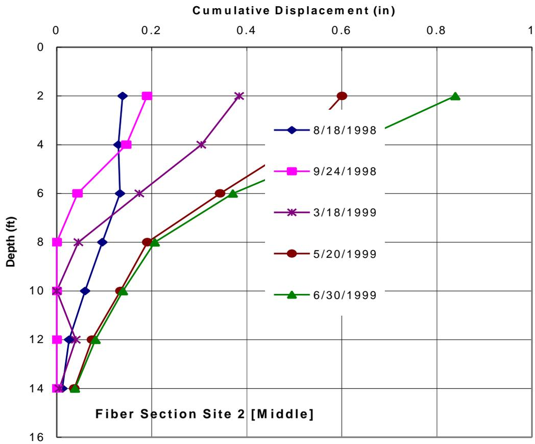
**Figure D-5: Readings of the middle inclinometer in fabric section 2**
