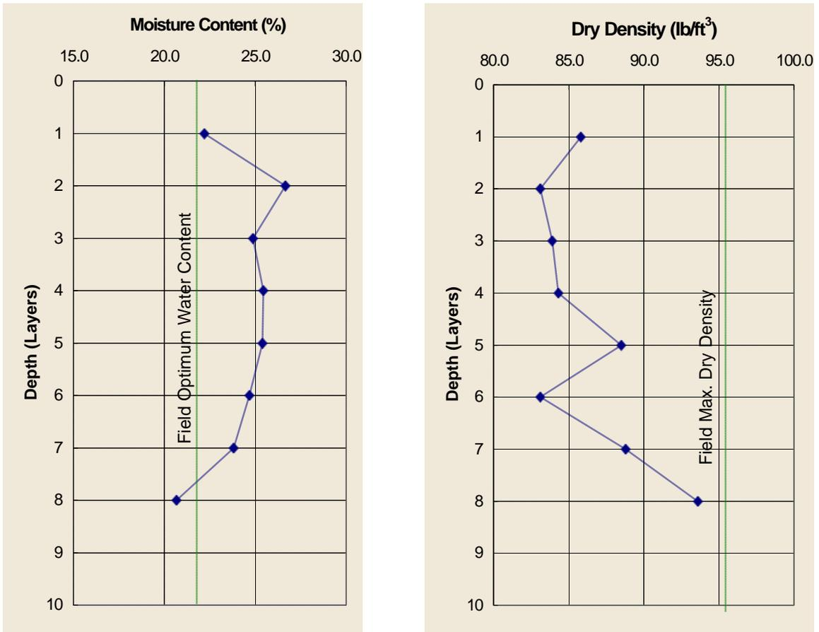
Figure A-4. Field measurements of moisture and density in section 213
