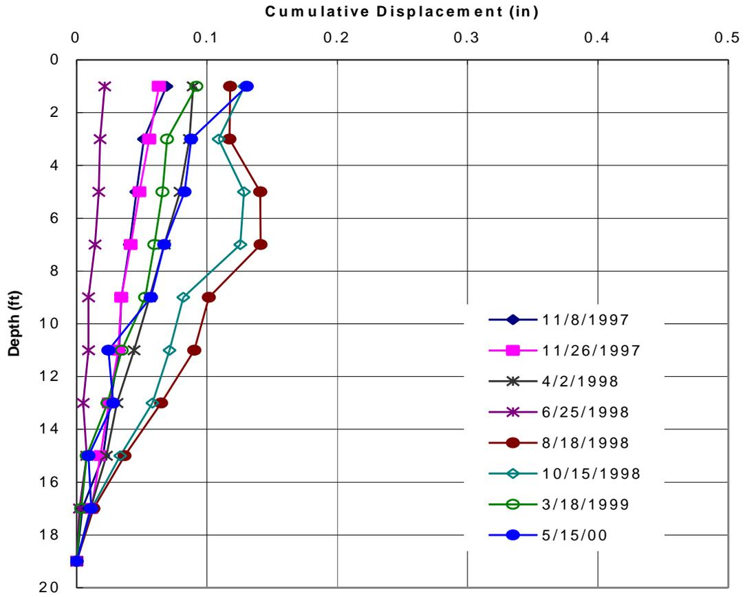
Figure C-8: Top inclinometer readings in section 224 [soil-fiber mix]
