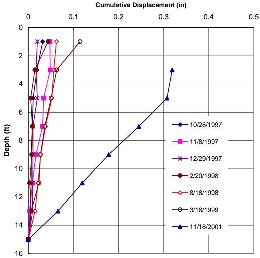
Figure C-15: Middle inclinometer readings in section 244 [soil only]
