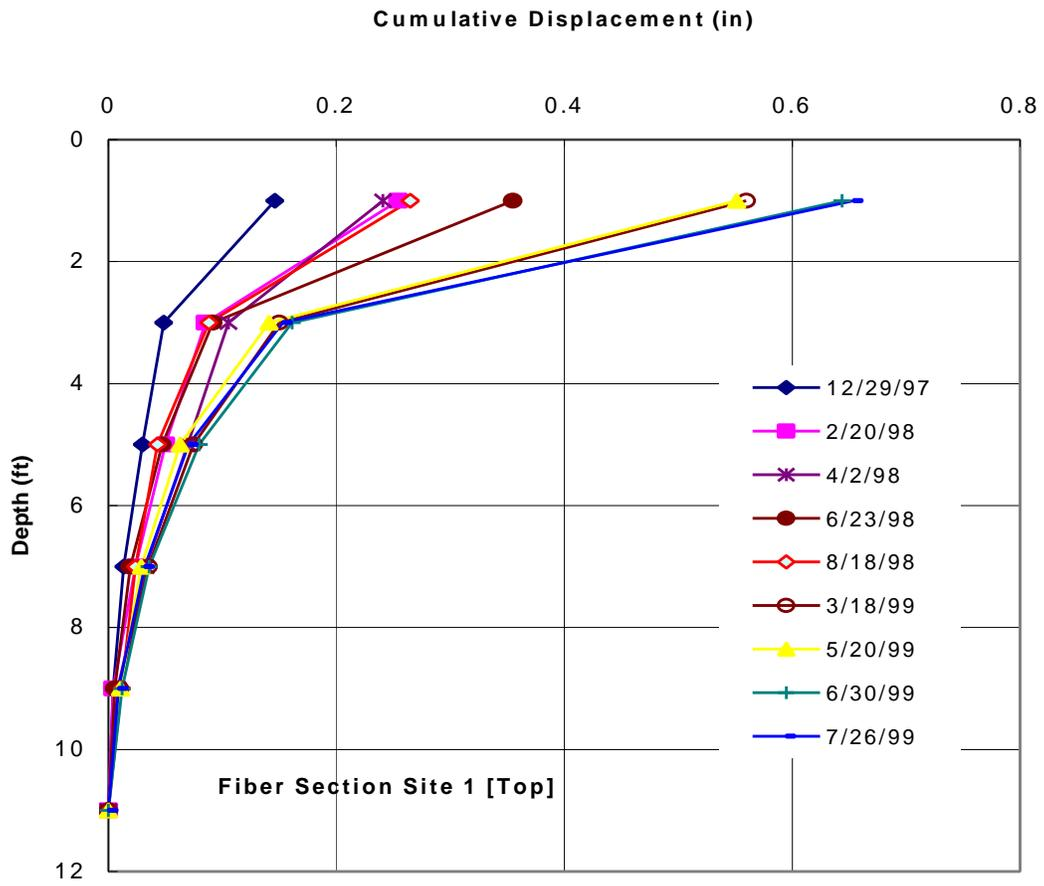
**Figure D-1: Readings of the top inclinometer in fabric section 1**
