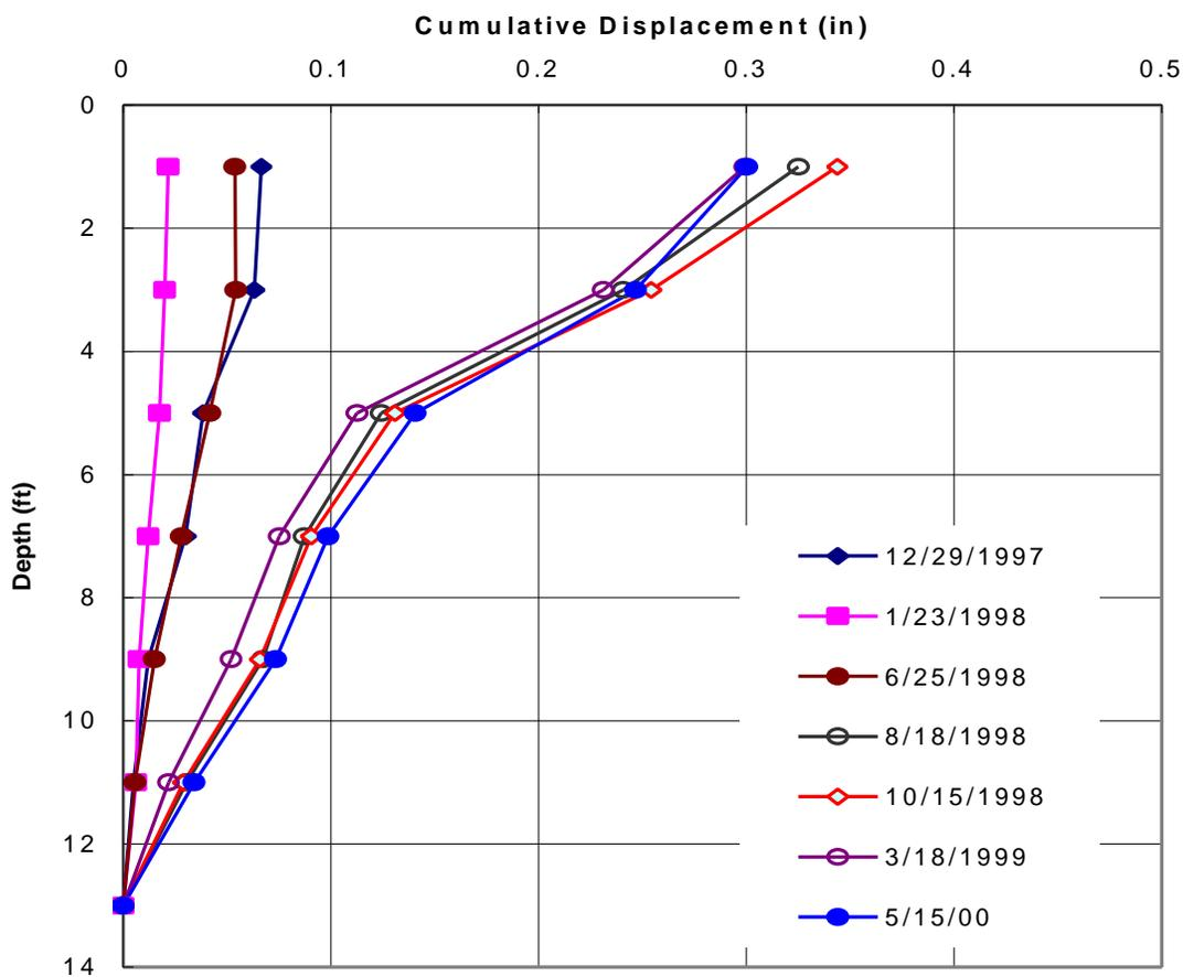
Figure C-12: Middle inclinometer readings in section 242 [soil only]
