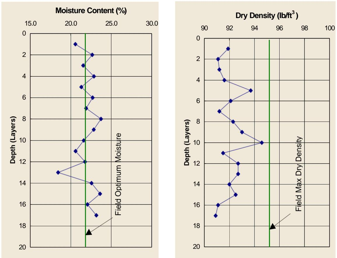
Figure A-2. Field measurement of moisture and density in section 132
