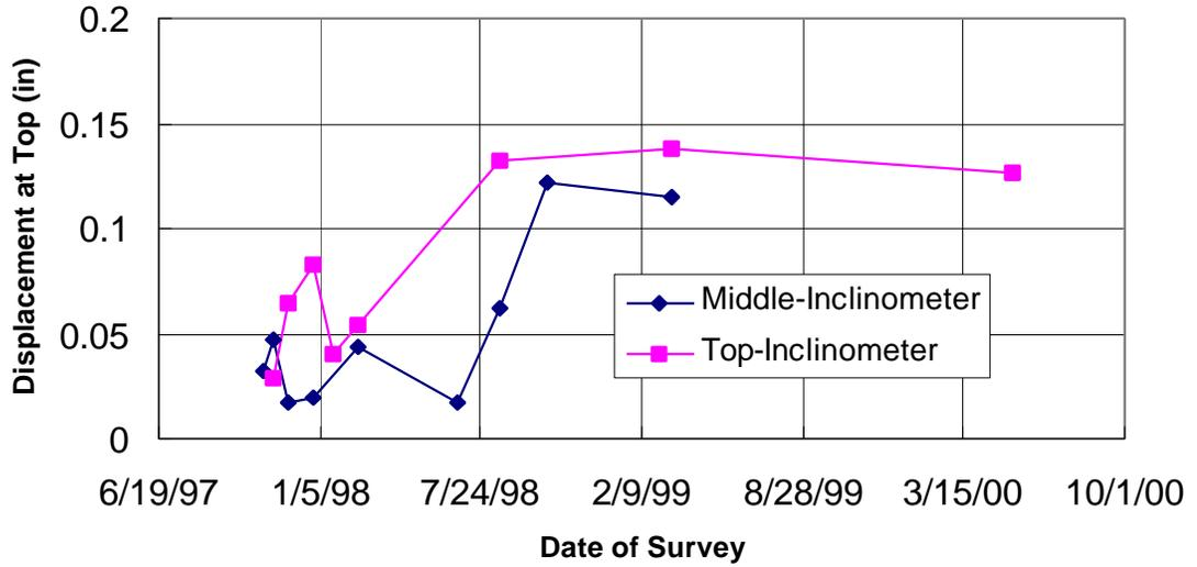
Figure C-16: Time deformation of the inclinometers, section 244
