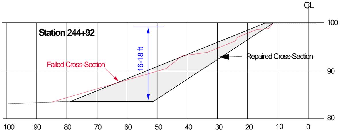
Figure A-7. Typical cross-section of the slope in section 244
