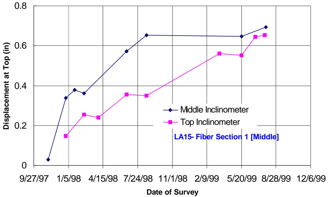
**Figure D-3: Time-deformation readings in fabric section 1**
