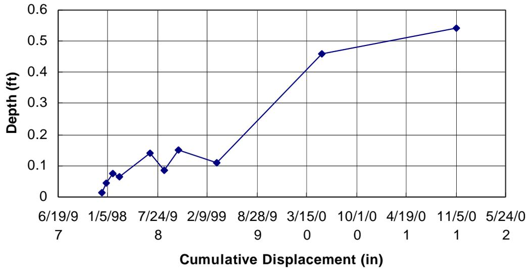
**Figure C-7: Time deformation at middle inclinometer, section 213**
