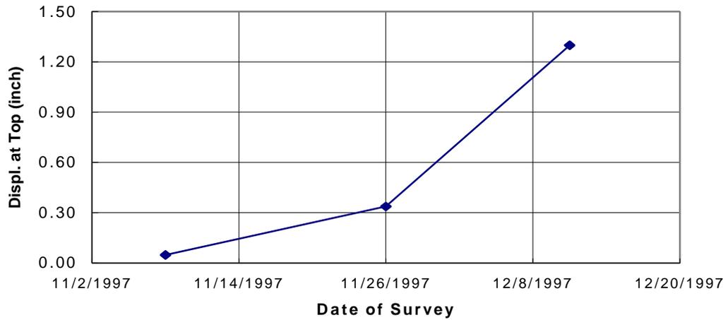
**Figure C-3: Time-deformations of the middle-inclinometer in section 132**
