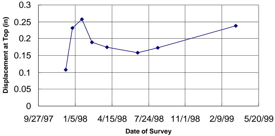
**Figure C-6: Time deformation at top inclinometer, Section 213**
