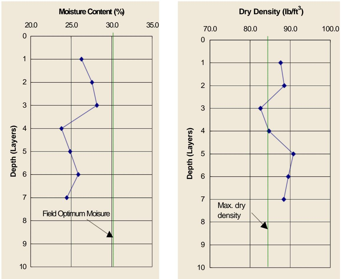
Figure A-8. Field measurements of moisture and density in section 244
