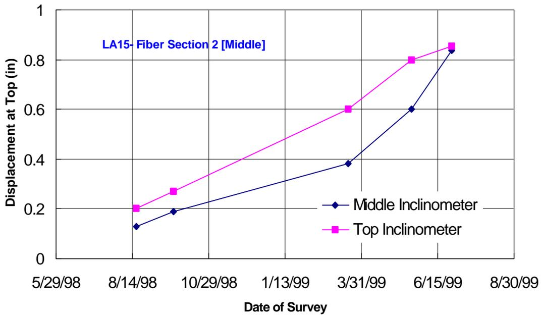
**Figure D-6: Time deformation readings in fabric section 2**
