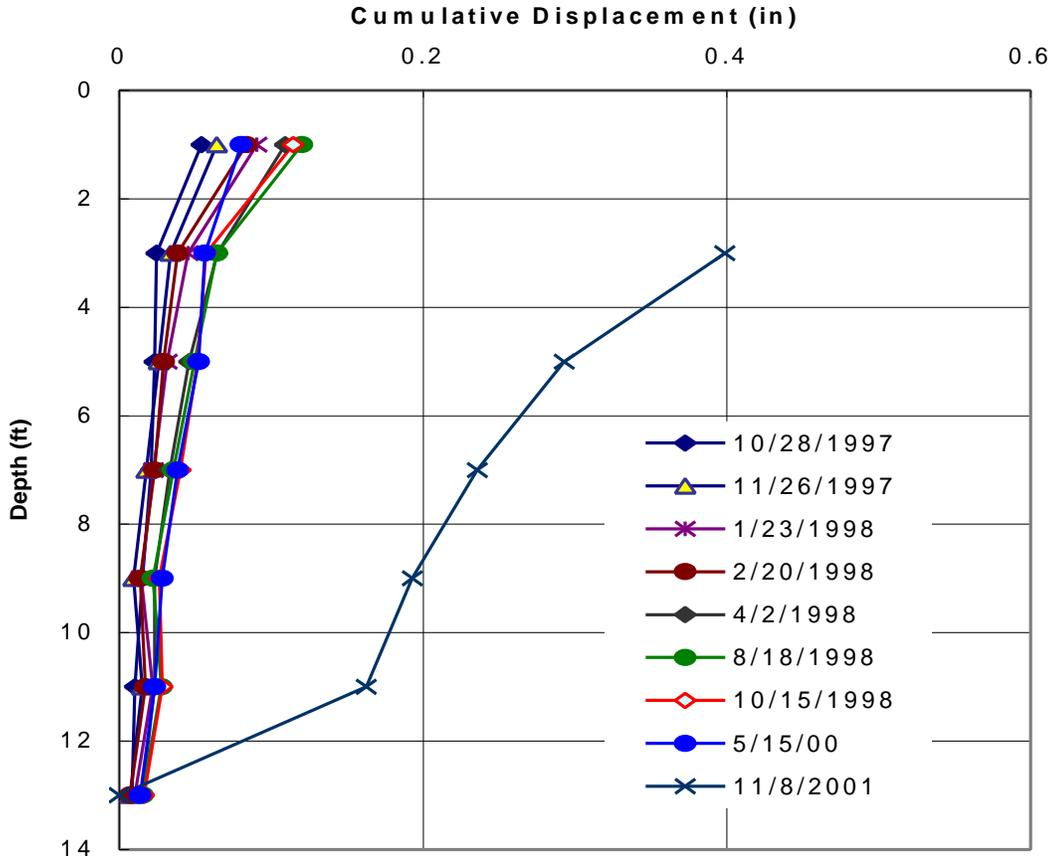
**Figure C-9: Middle inclinometer readings in section 224 [soil-fiber mix]**
