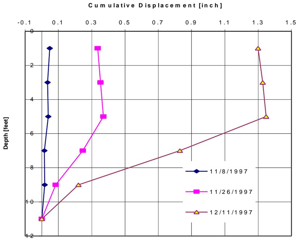
**Figure C-2: Middle-inclinometer readings in section 132 [soil-fiber mix]**
