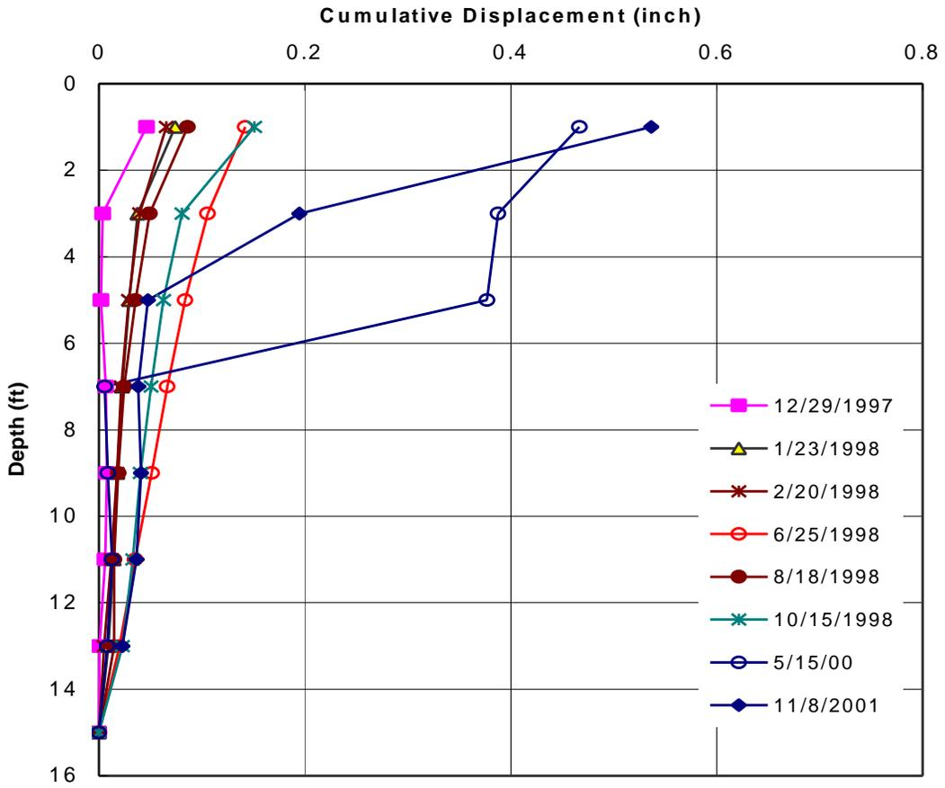
Figure C-5: Middle inclinometer readings in section 213 [soil-fiber mix]
