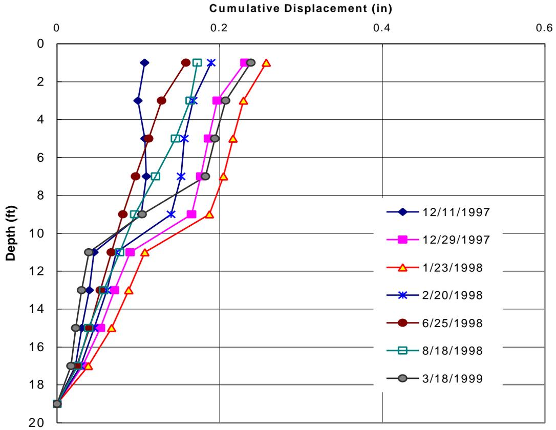
Figure C-4: Top inclinometer readings in section 213 [soil-fiber mix]
