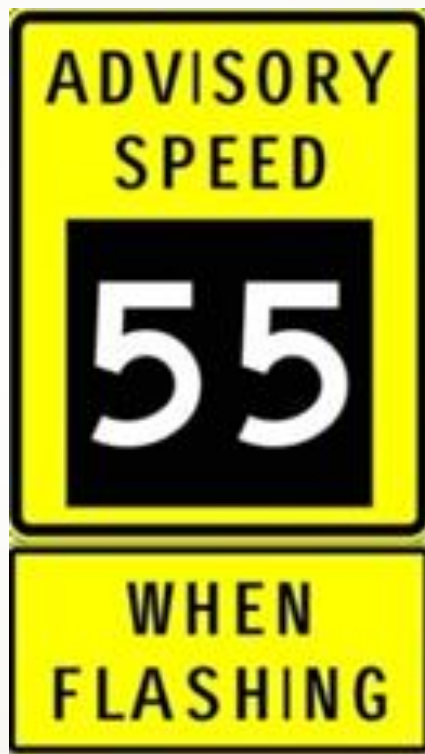
MoDOT variable advisory speed sign
